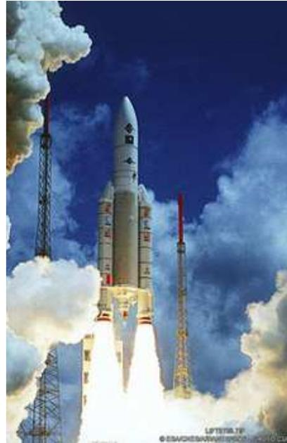
Exploded 37 seconds after takeoff - the reason was an overflow in a conversion of a 64 bit floating point number into a 16 bit integer.
